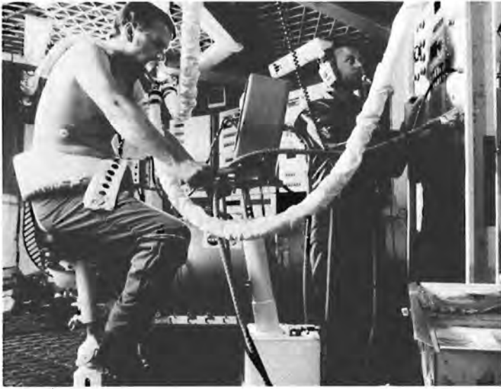
A Martin Marietta aerospace test engineer, wired with heart-rate measuring electrodes and breathing through a metabolic analyzer hose, rides an ergometer, a device resembling a stationary bicycle, in a full-scale Orbital Workshop mockup. Martin Marietta designed and produced equipment for this experiment to enable physicians on the ground to measure oxygen consumption, body temperature, heart rate, and blood pressure during Skylab missions. The engineer on the right checks a display panel to see that the participating engineer does not exceed predetermined physical limits.—Martin Marietta photo.
