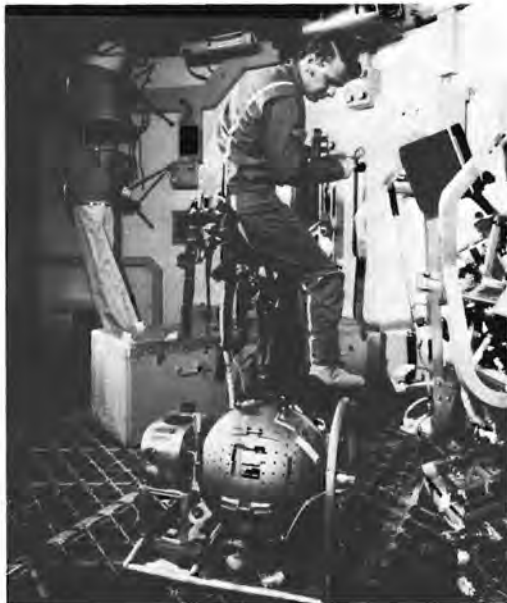
A Martin Marietta aerospace test engineer, wired with heart-rate measuring electrodes and breathing through a metabolic analyzer hose, rides an ergometer, a device resembling a stationary bicycle, in a full-scale Orbital Workshop mockup. Martin Marietta designed and produced equipment for this experiment to enable physicians on the ground to measure oxygen consumption, body temperature, heart rate, and blood pressure during Skylab missions. The engineer on the right checks a display panel to see that the participating engineer does not exceed predetermined physical limits.—Martin Marietta photo.
