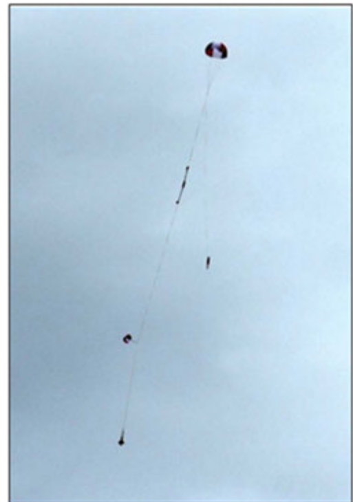
Rocket with drogue and main chute deployed.
